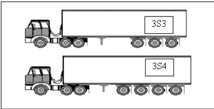
Figure 1-23. FHWA Class 10 — 6 or More Axles, Single Trailer
